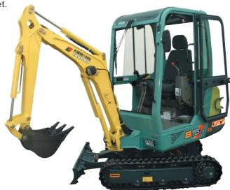
Use of a high performance engine and a modern hydraulic circuit: better productivity, less fuel consumption, less noise, less pollution.
